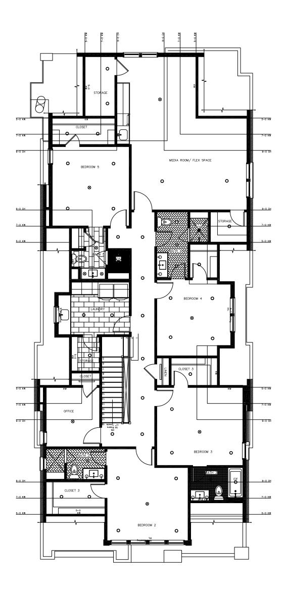
2ND FLOOR LIGHTING PLAN SCALE: <sup>1</sup>/<sub>8</sub>" = 1'
